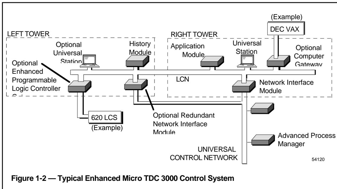
Figure 1-2 — Typical Enhanced Micro TDC 3000 Control System
