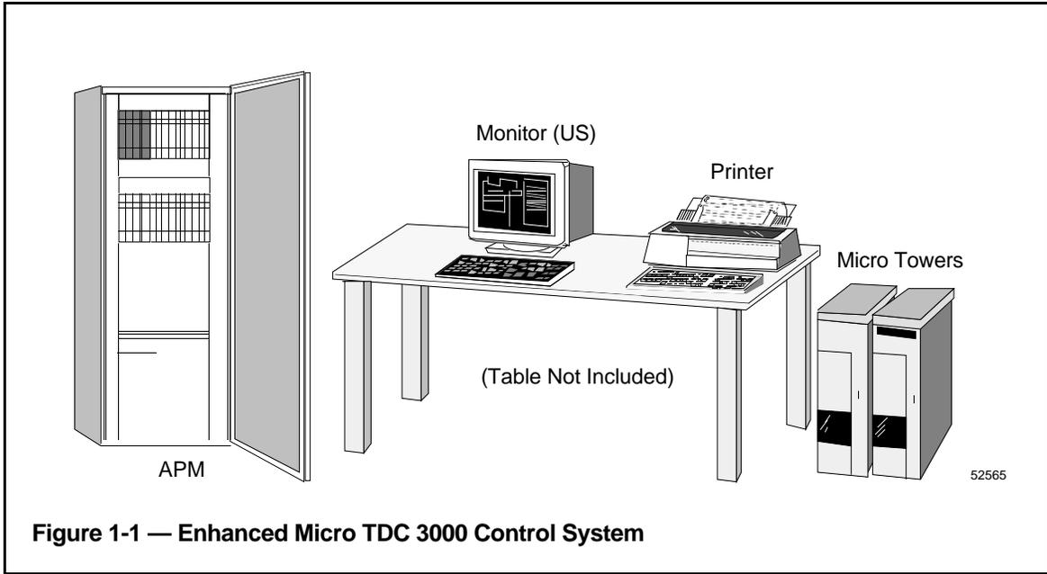
**Figure 1-1 — Enhanced Micro TDC 3000 Control System**
